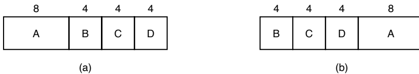
Figure 2-42. An example of shortest-job-first scheduling. (a) Running four jobs in the original order. (b) Running them in shortest-job-first order.
